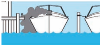
Blocked exhaust outlets.
