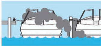
Another vessel's exhaust. CO from the boat positioned next to you can be just as deadly.
