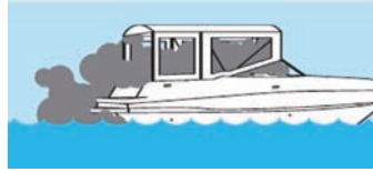
Inadequately ventilated canvas enclosures.
