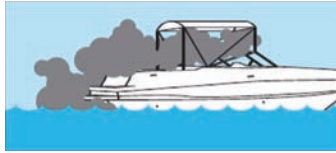
Exhaust gas trapped in enclosed places.
