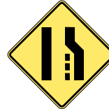
Lane Ends, Merge Left
