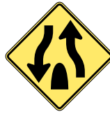
Divided Highway (Road) Ends
