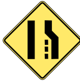
Lane Ends Merge Left
